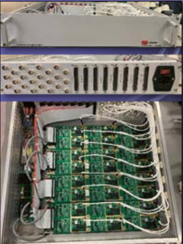
▼ Figure 5. The new AGA unit with 24 channels for high precision current measurements.
