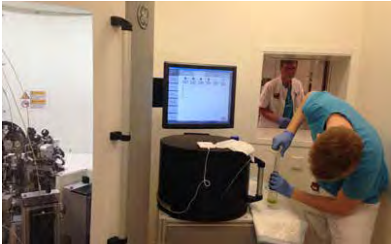
The hyperpolarized Pyruvate is drawn into a vial. The PET/MR scanner is right behind the hatch.
